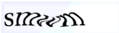
Figure 3: This CAPTCHA of 'smwm' obscures its message from computer interpretation by twisting the letters and adding a background color gradient [2].
